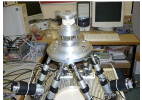
Fig. 1: The Dento-Munch, the world's first 6-DOF dental chewing simulator.
