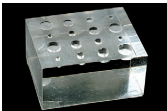
Fig. 2: Low-contrast phantom (seen from the side) with holes of different diameters (range 1.0-4.0 mm) and depths (range 0.5-2.0 mm).
